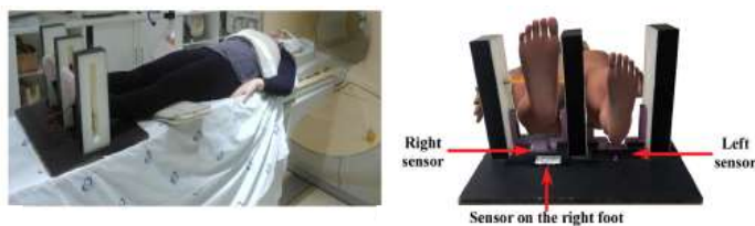
Figure 1 - The fMRI-compatible force measurement device.
